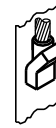
DETAIL 'G' TYPE "VF" MOLD CABLE UP TO STEEL NOTE: DIFFERENT DIES REQUIRED FOR ROUND & FLAT SURFACES.
